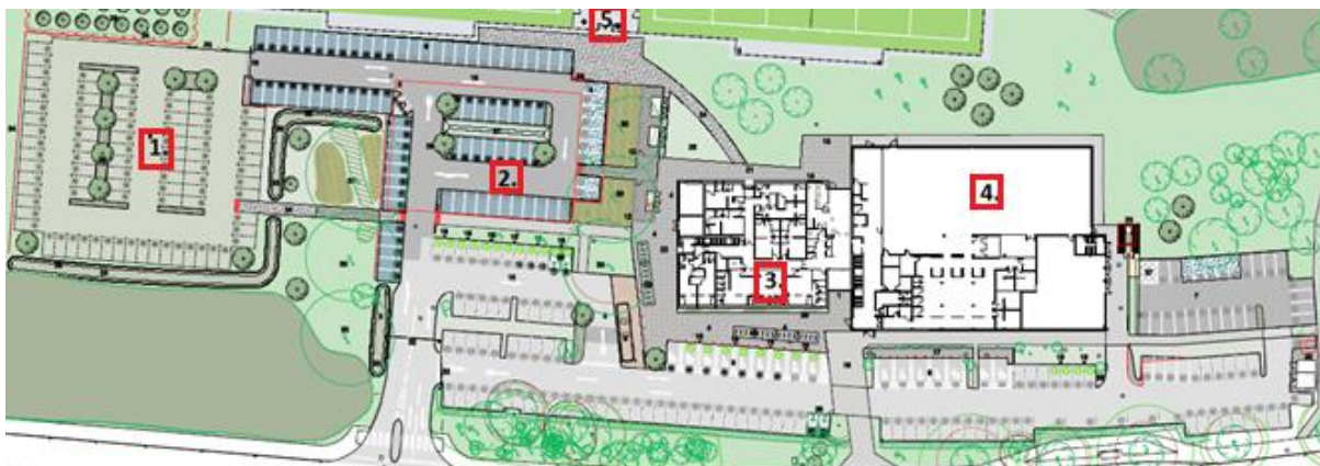
Proposed site layout – Overspill car parking to the left (annotated 1) , Car Park (2), Extension building (3) , existing Leisure Centre building (4) and 3G pitches (5)
