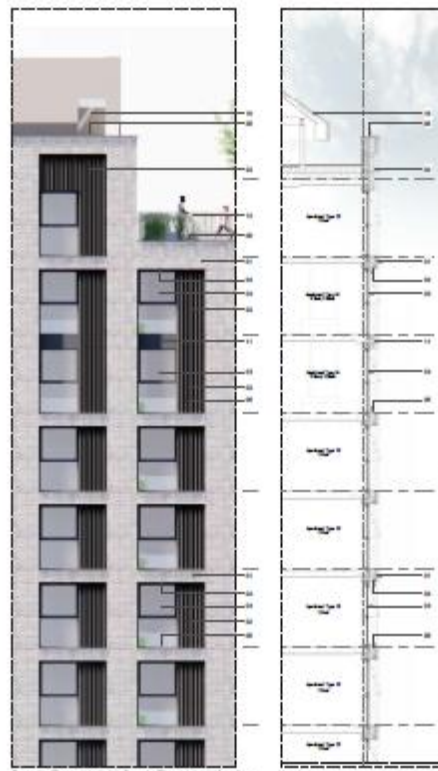
Step in Floor 14 & 15 South Elevation & Section
